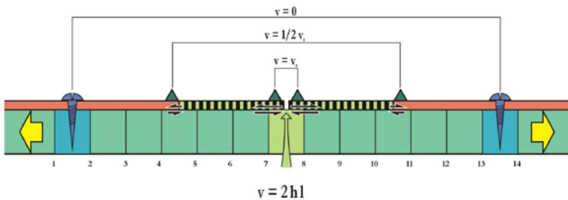
**Fig. 6. Relative speeds of the geodetic stations on the opposite sides of the ridge when the expansion of the basement is not noticed (explanation in text)**
